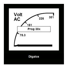
To configure the upper scale caption, connect J3 within 10 seconds after restart and disconnect it again. The device switches to programming mode. "Prog" appears in the display, followed by the upper scale caption, whereby the digit to be changed is shown as "x". Use J2 to select which digit is to be changed. Change the value of the digit with J1. Connect J3 again to save.
